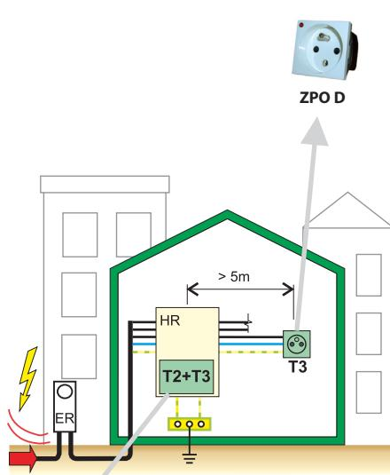
**$I_{max} = 40 \text{ kA}$  (8/20)/one conductor**
