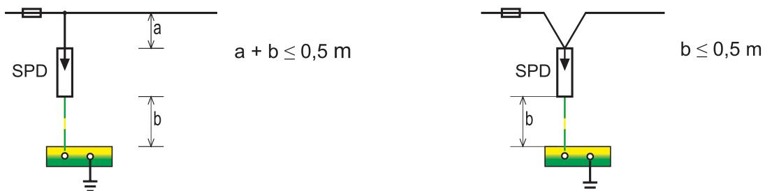
Important are also principles of conductors arrangement:
